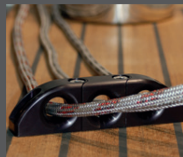
LO 18-35 as a triple version mounted on deck.
