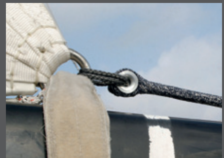
The LOOP® Connector on for an outhaul shackle.
