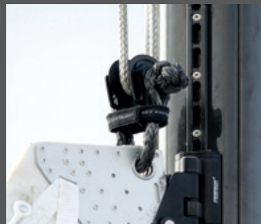
LOOP® Block 45 on a 55qm main on a modern 40ft. cruiser/racer.
