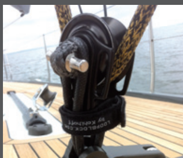
LOOP® Block LB-60-4BB on a Hanse 630 Race.
